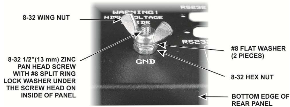
Figure 21. Installing the Rear Panel Ground Lug.
