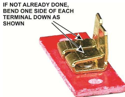
Figure 17. Preparing the Terminal Strip Board.
